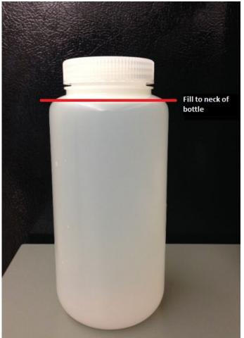
Tightly screw the lid back onto the bottle after collecting the sample.
